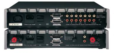
The 99 Pre-amplifier has an intelligent control system to communicate with all components connected via the 'Quad-Link' connector.
